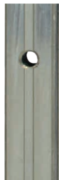
Rail with CZS coating - after 99 hours of salt spray test (according to DIN EN ISO 9227)
