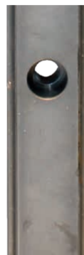
Rail with CTS coating - after 22 hours of salt spray test (according to DIN EN ISO 9227)
