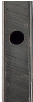
Rail with CCB coating - after 24 hours of salt spray test (according to DIN EN ISO 9227)
