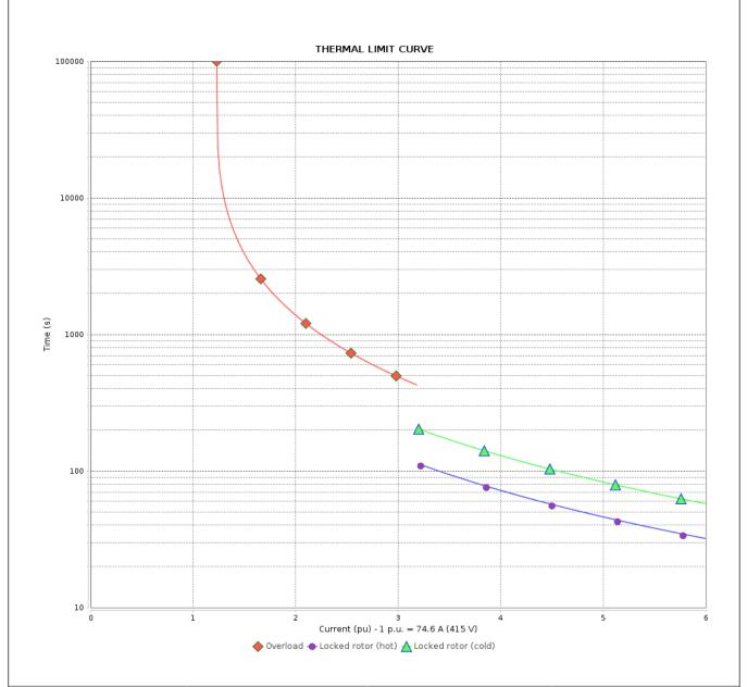
Performance : 415 V 50 Hz 8P Rated current : 74.6 A Moment of inertia (J) : 2.82 kgm<sup>2</sup> **LRC** : 6.0 Duty cycle : S1 Insulation class : 48.6 kgfm : F Rated torque : 200 % : 1.00 Locked rotor torque Service factor : 250 % Breakdown torque Temperature rise : 80 K Rated speed : 741 rpm Design : N Heating constant
