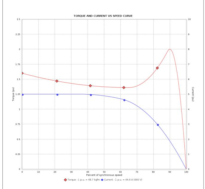
Performance : 380/660 V 50 Hz 8P Rated current : 77.5/44.6 A Moment of inertia (J) : 2.82 kgm<sup>2</sup> **LRC** : 5.0 Duty cycle : S1 Rated torque : 48.7 kgfm Insulation class : F : 160 % Service factor Locked rotor torque : 1.00 : 80 K Breakdown torque : 200 % Temperature rise Rated speed : 740 rpm : N Design
