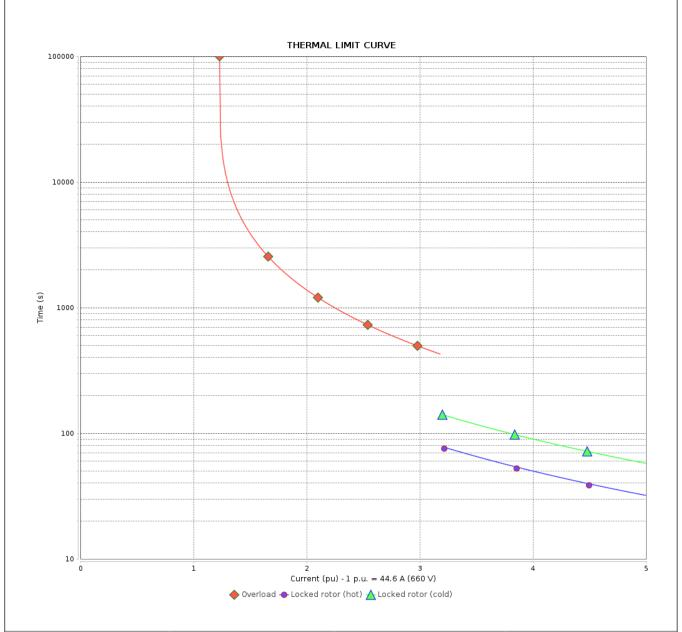
Performance : 380/660 V 50 Hz 8P Rated current : 77.5/44.6 A Moment of inertia (J) : 2.82 kgm<sup>2</sup> **LRC** : 5.0 Duty cycle : S1 Insulation class : 48.7 kgfm : F Rated torque : 160 % : 1.00 Locked rotor torque Service factor Breakdown torque : 200 % Temperature rise : 80 K Rated speed : 740 rpm Design : N Heating constant
