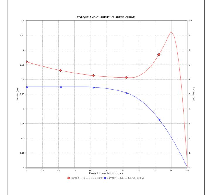
Performance : 400/690 V 50 Hz 8P Rated current : 75.4/43.7 A Moment of inertia (J) : 2.82 kgm<sup>2</sup> : S1 **LRC** : 5.5 Duty cycle : F Rated torque : 48.7 kgfm Insulation class : 180 % : 1.00 Locked rotor torque Service factor : 80 K Breakdown torque : 229 % Temperature rise : N Rated speed : 740 rpm Design
