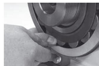
After mounting, the RIC should be checked at the unloaded roller.
