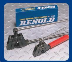
Renold's end-softened pin and spin rivet help to minimise downtime. All you need is a Renold pin extractor and you can disassemble Renold roller chain in seconds; no need to grind the head of the pin, no need for lengthy downtime.
