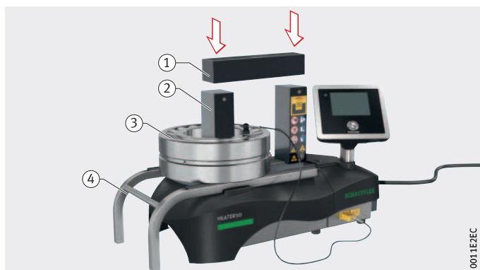
Figure 38 Rolling bearing lying flat, support ledge
